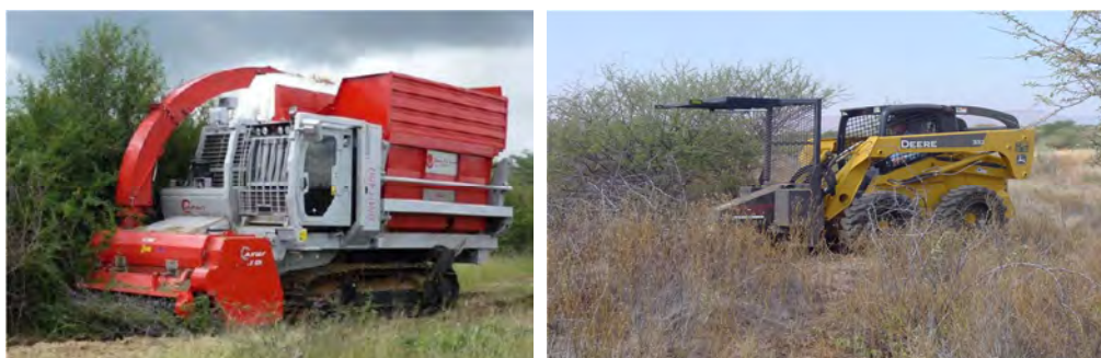
Figure 37: Track-mounted harvesters (left, [4.10]) and skid steer bush harvester (right, [4.11])
