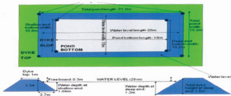
Figure 5: Plan view showing the pegging positions for a 300 m 2 pond
