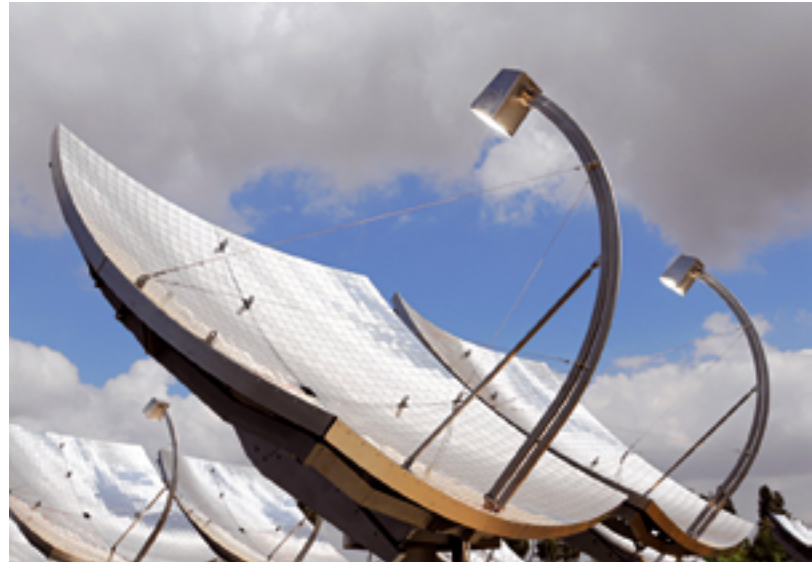
Modular and swivelling collectors generate both heat and electricity for homes.
