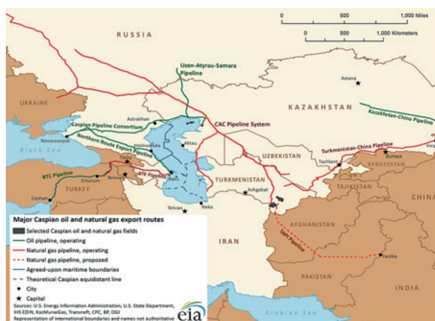
Figure 8: Major Caspian Oil and Gas Pipelines
