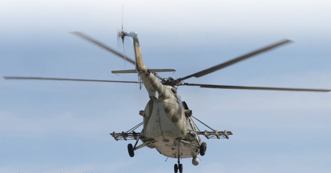
Military transport helicopter Mi-8 of the Armed Forces of the Republic of Belarus.
