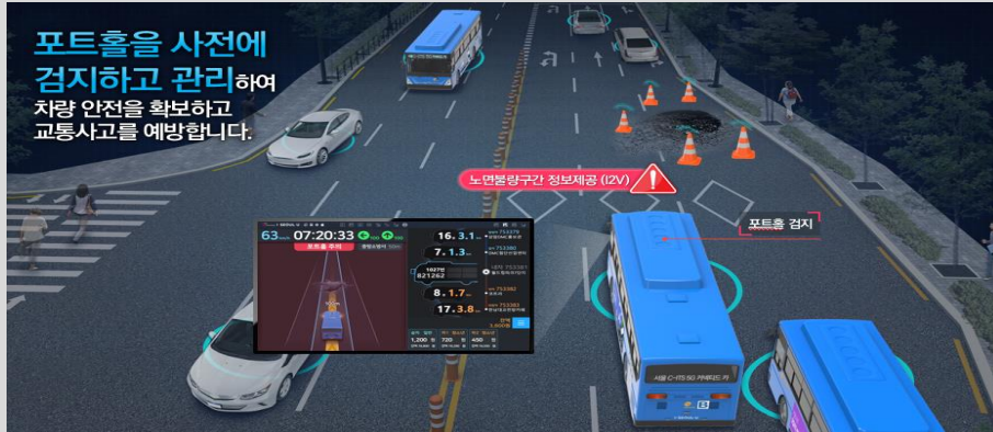
Pothole detection and transmitting photo evidence
