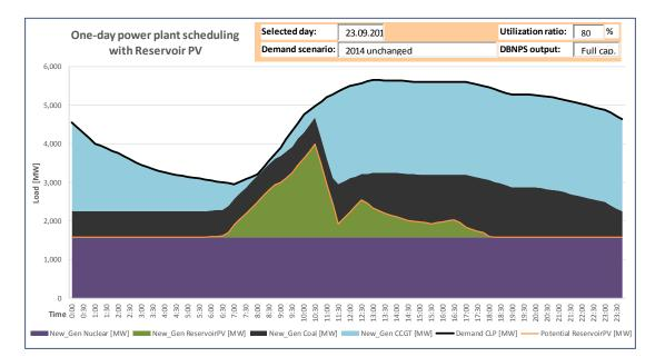
Figure 07: One-day power plant dispatching for 23.09. in "2014 unchanged" scenario with solar PV at 80% utilisation ratio (own compilation)
