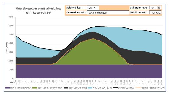
Figure 06: One-day power plant scheduling for a summer day (28.07.) in "2014 unchanged" scenario with solar PV at 80 % utilisation ratio (own compilation)
