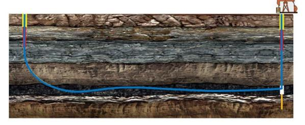
Figure 4. CBM mining technology using hydraulic fracturing
