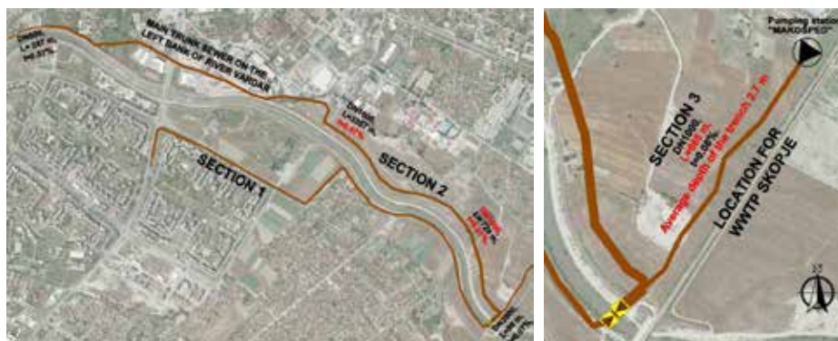
Figure 3-29 a) Sections 1 and 2 Trunk sewers on both river banks b) Section 3 Connection of the PS Makosped to the new main trunk sewer
