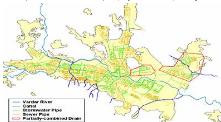
Figure 3-26 Existing storm drainage infrastructure
