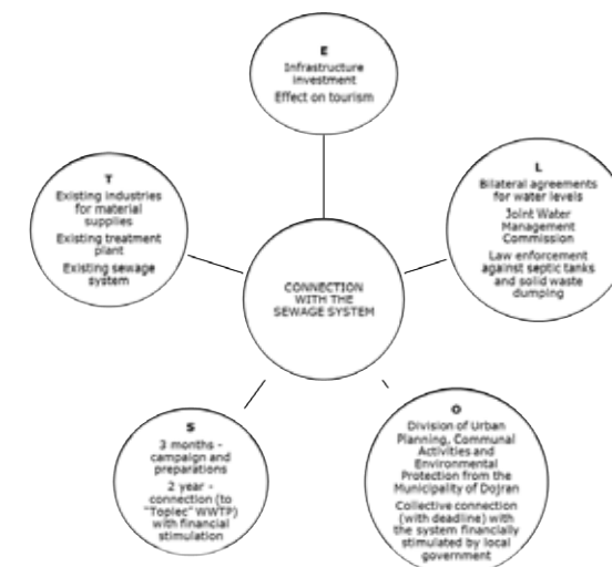
Figure 6-25 TELOS pre-feasibility analysis for connection with the sewage system for the Dojran/ Dorani lake
